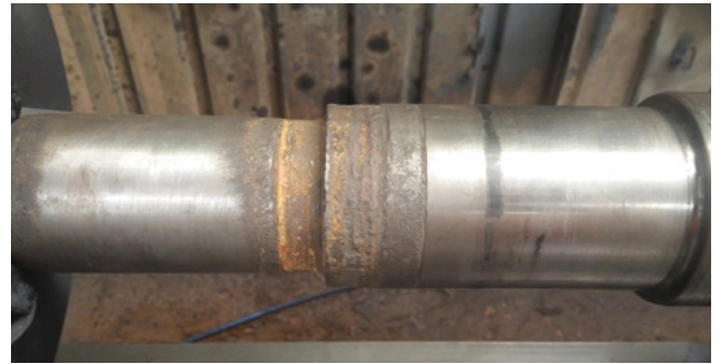
Shaft Before Thermal Arc Spray
