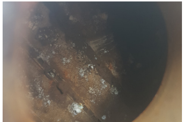
Radiator analysis showing stray current damage
