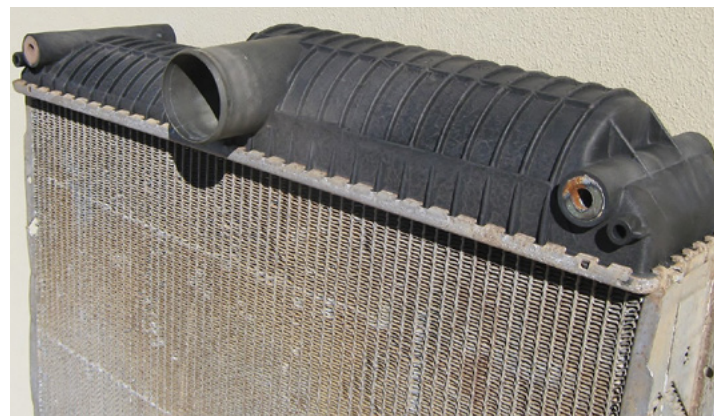
Removed OEM radiator
