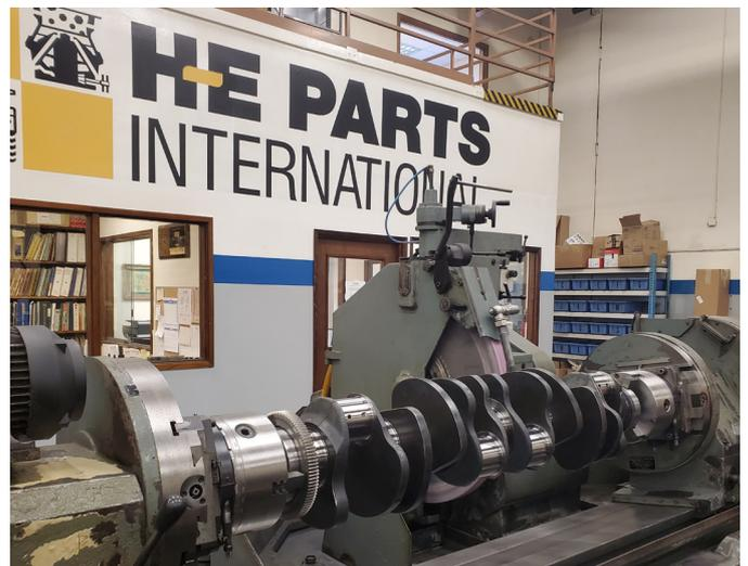
Crankshaft Set Up for Grinding
