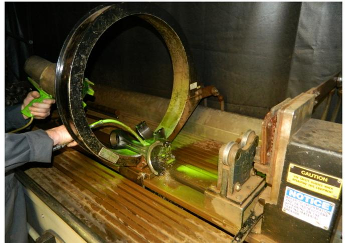
Connecting Rod Magnetic Particle Inspection (NDT)
