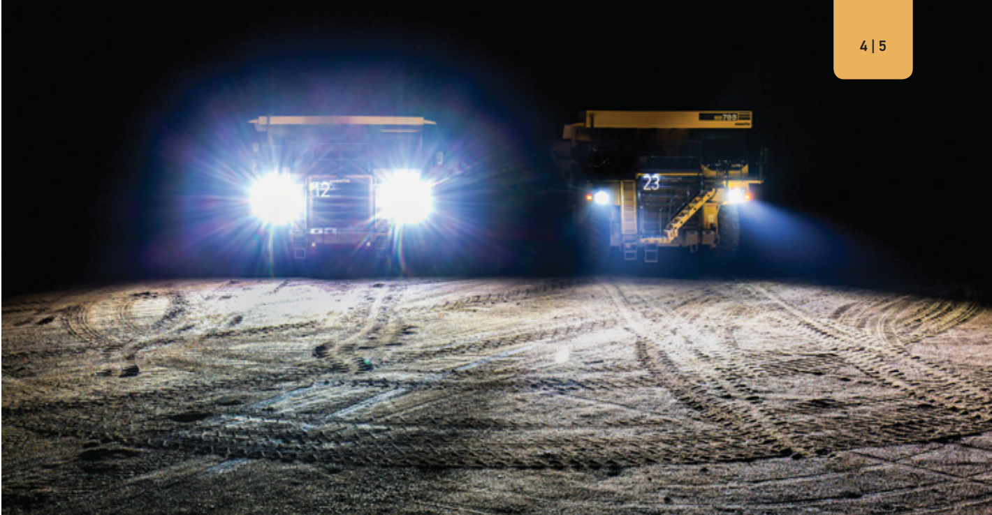
Traditional LED worklight vs. ZEROGLARE worklight
