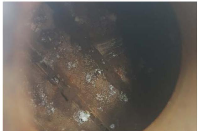
Radiator analysis showing stray current damage
