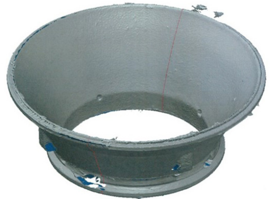
3D scanned worn OEM liners
