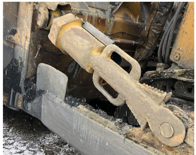
Ambidextrous D10T Tilt Cylinder on Dozer at Gold Mine in Nevada
