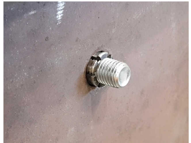
Nut locking mechanism on external side
