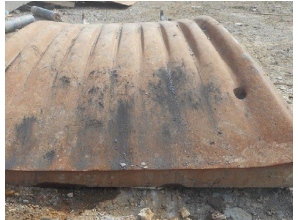
Worn OEM fixed jaw liner
