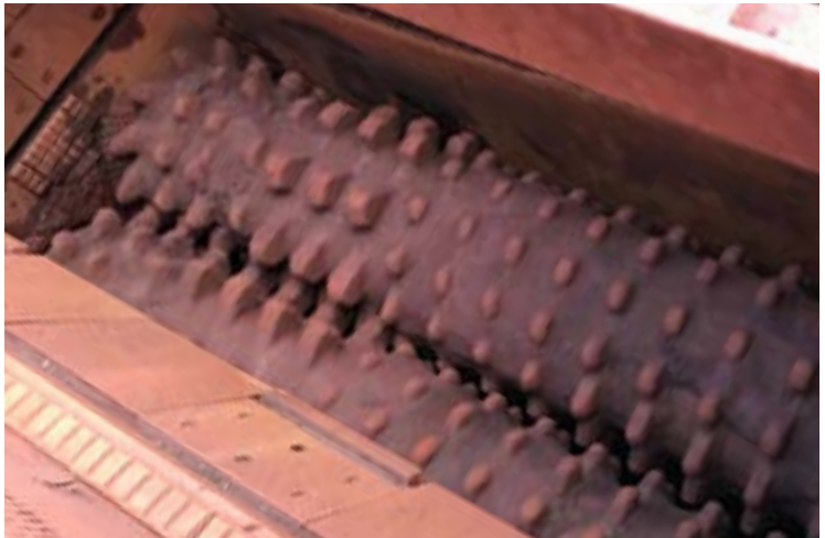
CME™ compatible replacement sizer segment teeth (left of centre) vs. OEM supplied teeth
