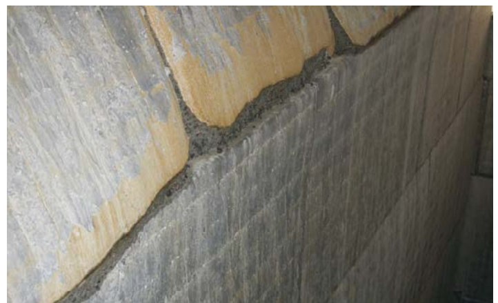
Standard overlay plate after 1300 hours.
