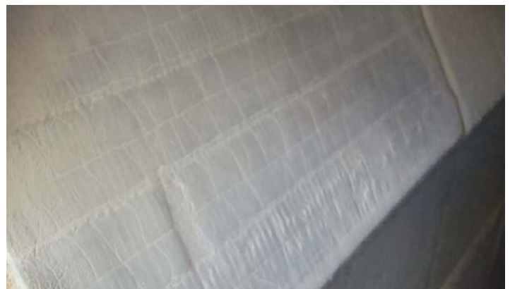
CME™ overlay wear liners after 3500 hours and 8.3 million tonnes
