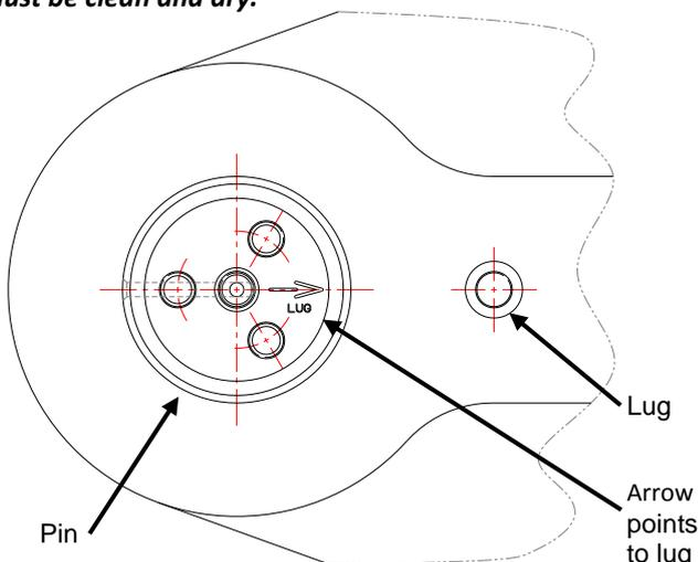
4. Loosely fit the collets to the chassis and axle housing bores. Tap the collets inwards, using a soft-faced hammer to engage the taper on the pin.
